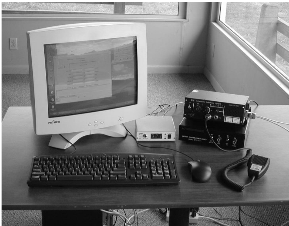
Figure 1 Typical Display Acquisition Terminal Unit setup
